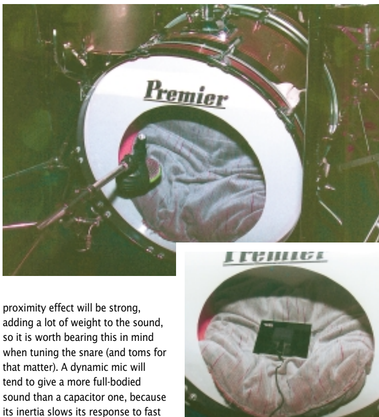
Two approaches to miking the bass drum: a dedicated mic on a stand (top), and a PZM on the cushion inside the drum (bottom).
